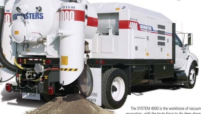
excavators, with the brute force to dig deep down with air, exposing utilities in even the hardest soils without harming them.
